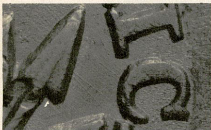
1853 $2½ Gold: Genuine. Pattern of heavy and light die polish marks between arrow heads and bottom of IC of AMERICA.
