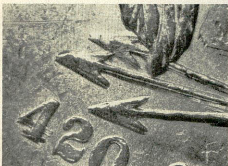
1878-S Trade Dollar: Genuine. Doubled die reverse displays doubling on all lettering. Doubled dies in the Trade Dollar series are relatively common. ANACS has recorded five different doubled dies, and several more varieties no doubt exist.
