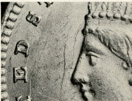
1874 $1: Genuine. Diecracks connecting many of the letters. The marks immediately in front of Liberty's face are clash marks, a common occurrence on all coins from all Mints.
