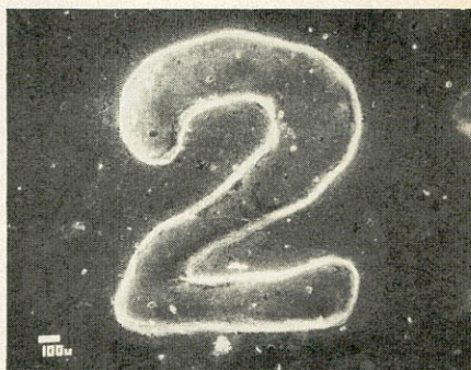
1921-S 50¢, altered from 1941-S, 50-X, back-scatter and secondary beam, 8° tilt.
