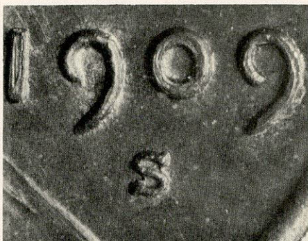
1909-S 1c: Counterfeit. Tool marks on the digits in the date.
