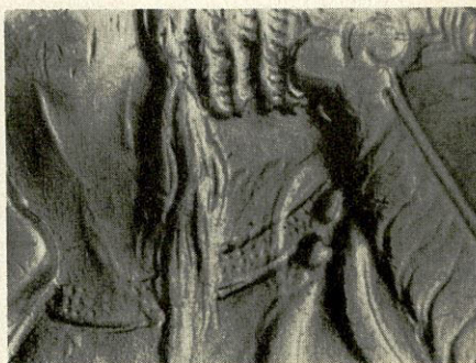
1913 $5 Gold: Genuine. Clashmarks on the neck, corresponding to the feathers of the eagle's wings on the reverse, are often mistaken for counterfeit die tooling.
