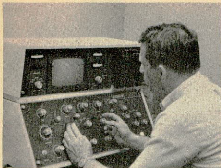
The image of a coin is flashed on the viewing screen of the scanning electron microscope. The SEM allows the authenticator to spot alterations.
