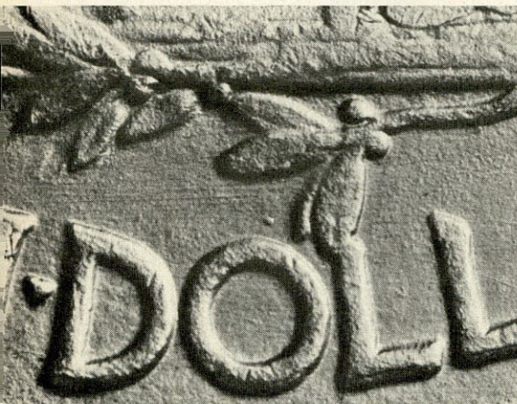
Counterfeit of a counterfeit with depressions and loss of detail.
