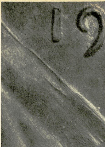
1909-S 1c: Counterfeit. Tool marks on the front of the coat.
