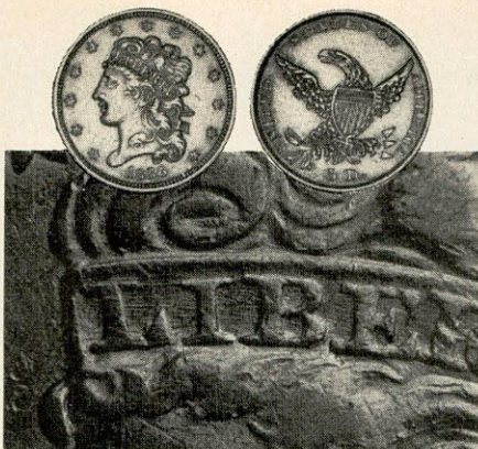
1836 $5 Gold: Genuine. The pattern of fine horizontal die polish marks on the headband is diagnostic of this die.
