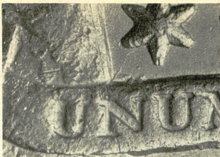
1806 $5 Gold: Genuine. Rust pitted dies left some lumps of metal on the top edge of the ribbon at the back of the eagle's neck. A die crack appears between that point and the star.
