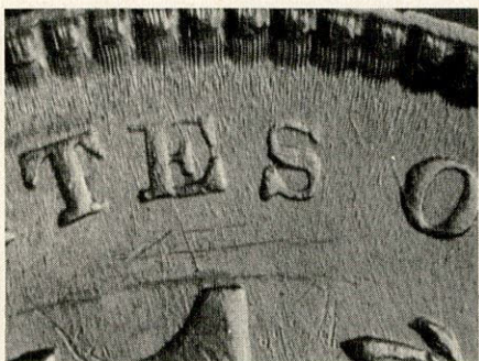
1853 $1: Genuine. Very worn die, resulting in weak letters and some die gouge marks (the raised lines in and below the E of STATES and left of O in OF.
