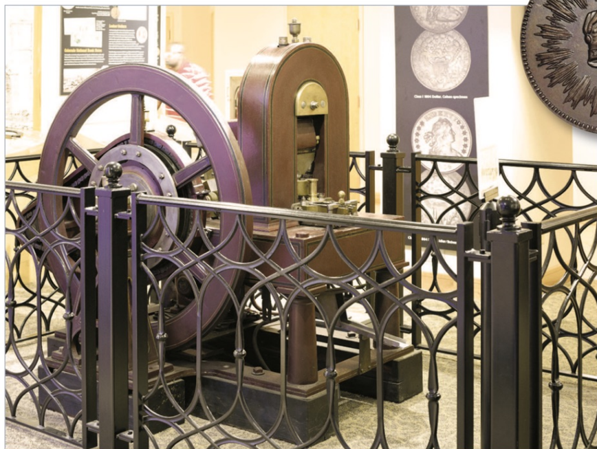
▲ THE FIRST STEAM-POWERED COIN PRESS used by the U.S. Mint awes guests at the ANA Money Museum. It produced coinage from 1836-75.
