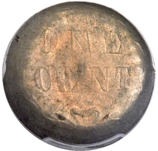
1859 Indian Head cent die cap error. A planchet became affixed to the obverse die face after being struck. Repeated strikes molded the stuck coin onto the obverse die to the point where it formed over the sides of the die neck creating a "bottle cap" appearance. Any coins struck by this die cap would have a normal reverse with an obverse looking like a distorted mirrored image of the reverse design. The reverse of this stuck coin functioned as an obverse coin die.
