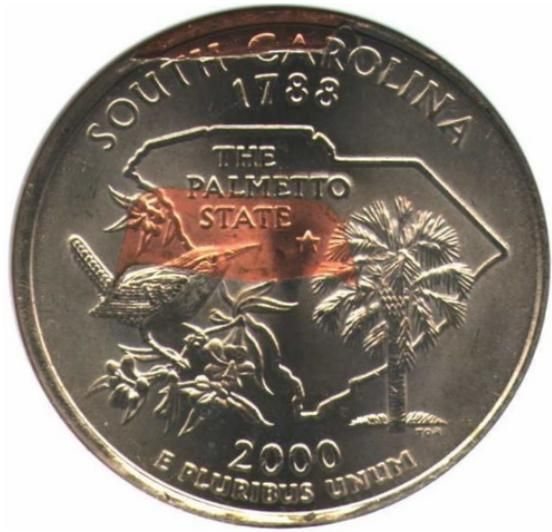
2000-P South Carolina statehood quarter reverse missing partial clad layer. Copper underneath is showing.
