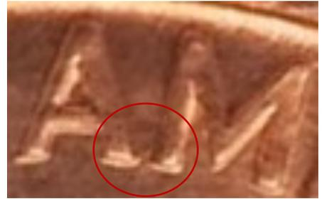
1998-2000 Lincoln cents with "Wide AM" reverse. For these three years, circulation-strike cents were mistakenly struck with dies usually prepared for proof coins, based on the separation between the bases of both letters. The middle photo is the common, Close AM. Wide AM coins are much harder to find, especially for 1999.
